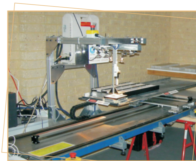
CSIRO's HyLogger using HyChips technology to quickly determine regolith mineralogy.
